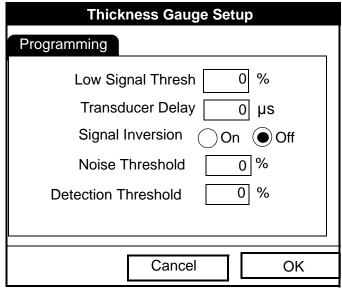
Figure 115: Thickness Gauge Programming Window
